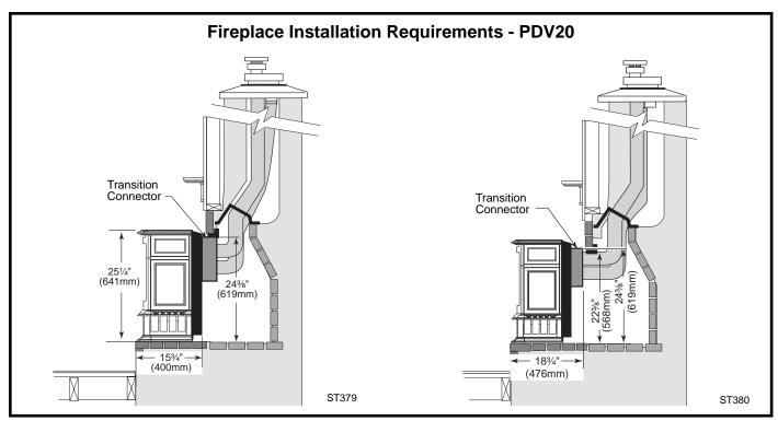
Fig. 36 PDV20 minimum lintel height for flush or forward placement.
